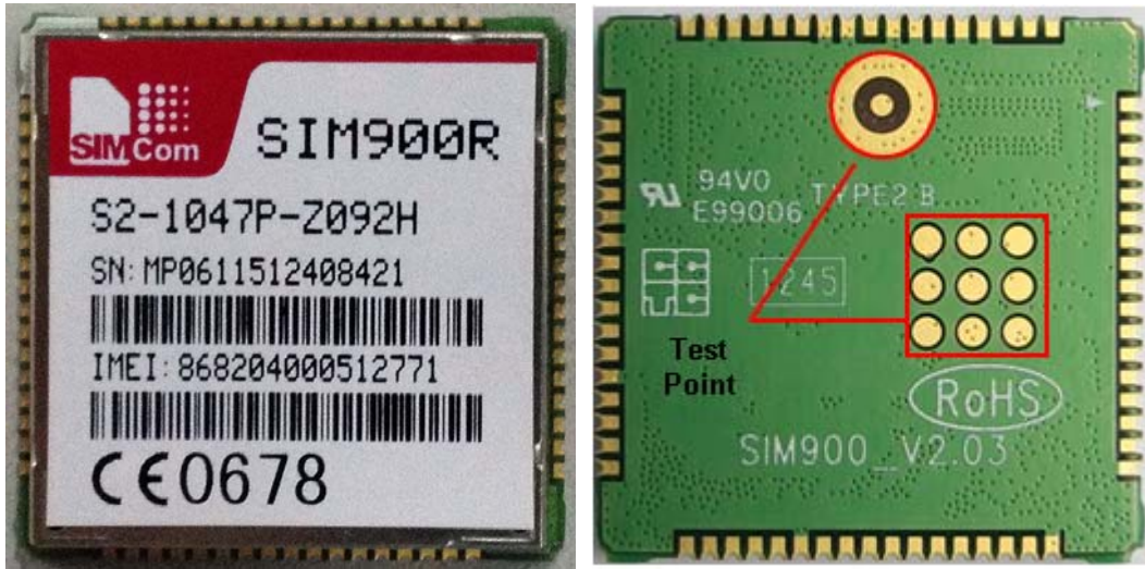
Figure 38: Top and bottom view of SIM900R
