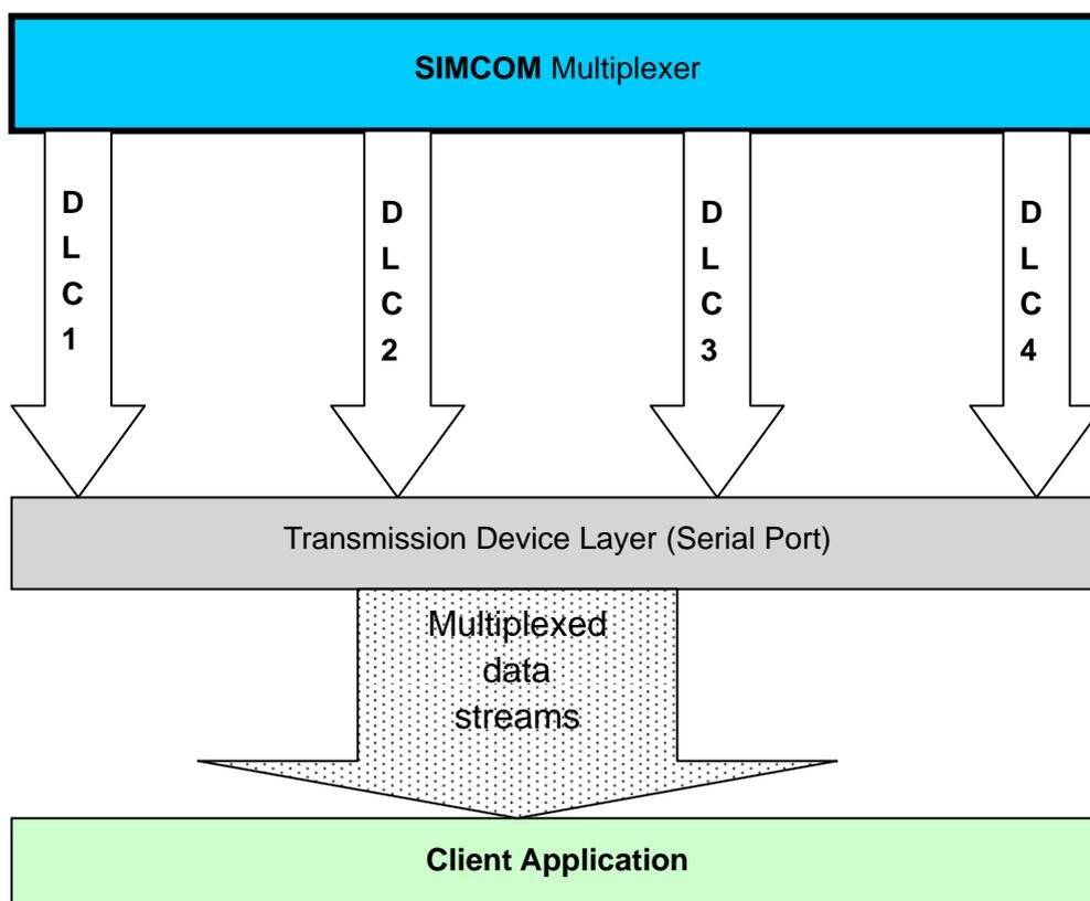
SIMCOM Multiplexer is established upon system transmission device layer (Commonly serial port). Data streams are addressed with DLCI value and encapsulated in frames based on GSM 0710 protocol (Chapter 2, SIMCOM Multiplexer Protocol) and transmitted through interface provided by transmission device layer.
